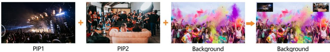
The video switcher supports two groups PIP or one POP. When press PIP1 or PIP2 button, there will be a small image display on the top left corner of PVW window. Press the Menu knob and choose the PIP setting interface, user can set parameters including position, size, border etc. Press ON AIR button next to PIP1 and PIP2 to put the PIP into effect on PGM.
