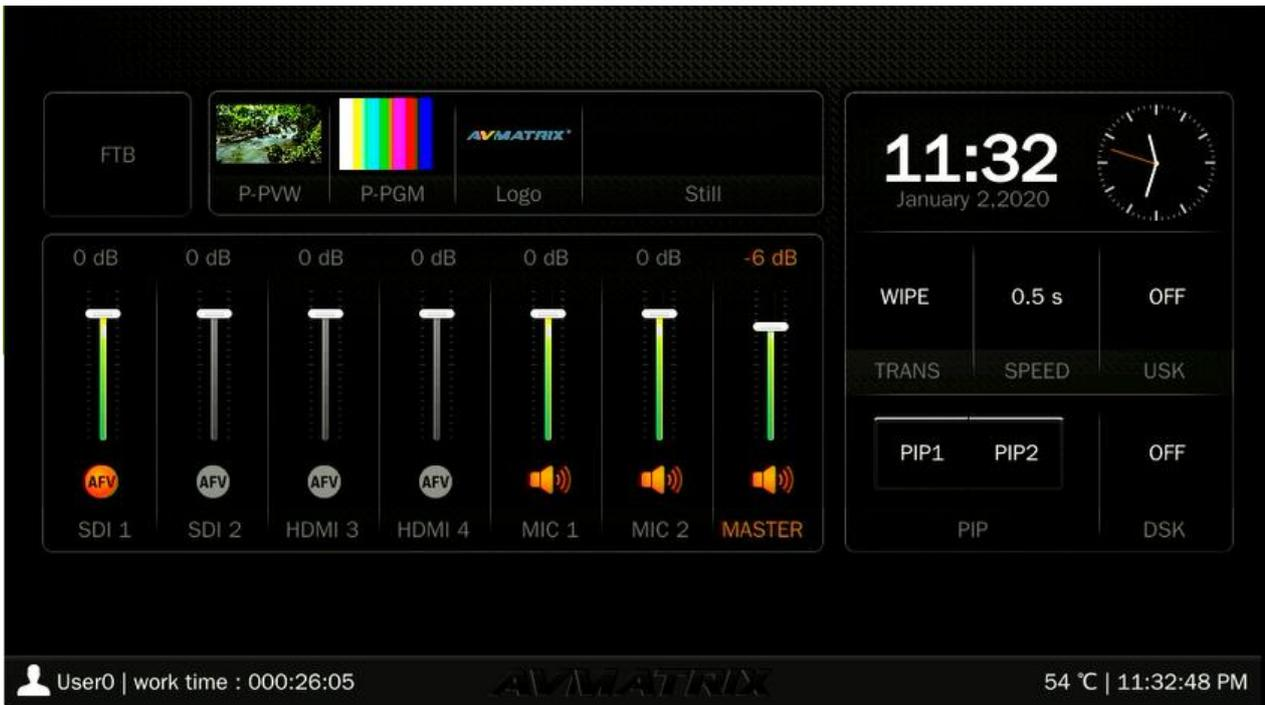
The information of user name, working time, USB connection, CPU working temperature, system time keeps displaying in the bottom of the Status/Menu page.
