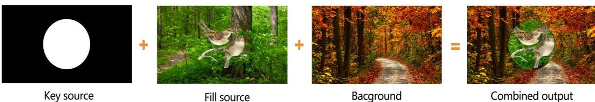
Luma keys provide a way to composite a Text clip over a background clip based on the luminance levels in the video. Turn on the Luma Key, a color from the key source will be removed, revealing another background image behind it.
