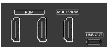
PVS0403U has 4 output interfaces. They are default as 2PGM Out, Multiview Out and USB Out. All the 3 outputs also can be defined as an AUX OUT from SDI1, SDI2, HDMI3, HDMI4, PVW, PGM, Clean
